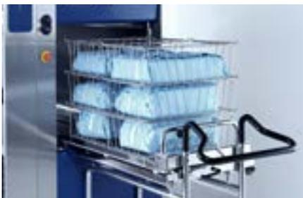
*Manual loading/unloading of wire baskets. Also using optional loading module(s) to process containers.*
