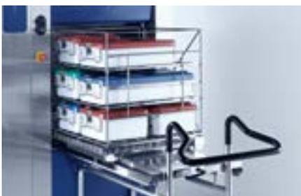
*Manual loading of containers or various packs using a loading platform and loading module on a loading trolley.*
